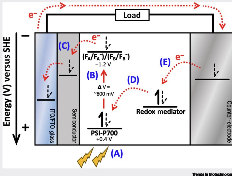
Figure 1. Dye-Sensitized Solar Cells (DSSCs Are an Emerging Third-Generation Photovoltaic Technology). Solar photonic energy is converted into electronic energy that is capable of performing work in a manner similar to that of biological photosynthesis. Abbreviations: FTO, fluorine-doped tin oxide; ITO, indium-tin oxide; SHE, standard hydrogen electrode.
